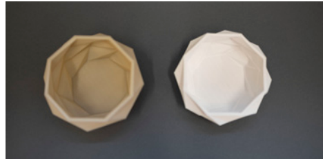
Examples of printed part shrinkage after drying.
